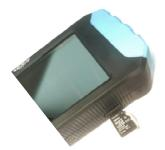
When recording battery pack data or upgrading battery pack software, please insert the TF memory card into the TF slot at the bottom of the PBA.
