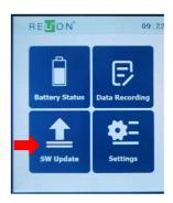
♦ An on-screen keyboard will appear when SW Update is selected, allowing you to input password. (default password is 1111)
