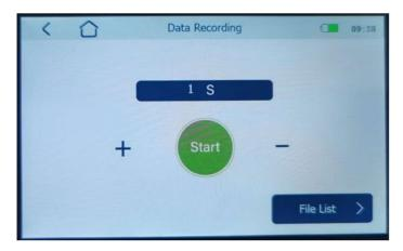
♦ Data recording interval can be changed by clicking + or -, the range is 1~99 Second.
