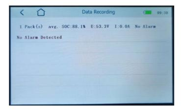
Battery Bank Information When the PBA is connected to the battery, the corresponding battery information will be displayed:
